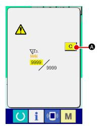
When the count-up condition is reached during sewing work, the count-up screen is displayed and the buzzer beeps. Press CLEAR button C to reset the counter and the screen returns to the sewing screen. Then the counter starts counting again.
