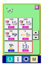
2-step stroke position used in the user's pattern can be set with memory switch 1026.
