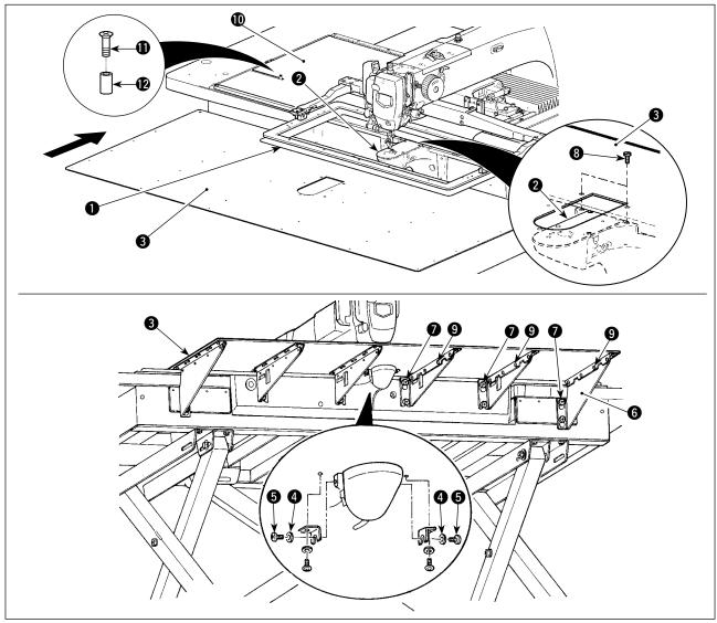
1) Move the cloth feed base to the rear and place throat plate auxiliary cover (asm.) (3) from between lower plate (1) and throat plate (2).
