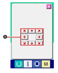
Lower the presser, and input the move direction with DIREC-TION key **(B**).
