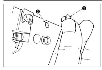
When thread is caught at top end ① of the thread clamp, thread clamp becomes incomplete and sewing trouble at the sewing start will be caused. Thread waste and lint are likely to accumulate in the sections which are shown in the circles. The sections should therefore be periodically cleaned by removing the throat plate and by blowing air through hole 3 by removing rubber plug 2.
