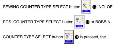
corresponding counter type select screen is displayed. On this screen, the counter type can be selected individually.
