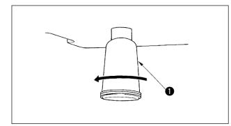
When polyethylene oiler ① becomes filled with oil, remove polyethylene oiler ① and drain the oil.
