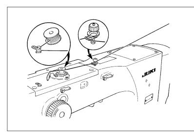
Thread the bobbin winder and wind the bobbin thread onto the bobbin as illustrated in the figure.
