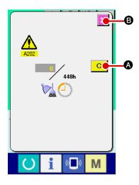
When the designated inspection time is reached, the warning screen is displayed.
