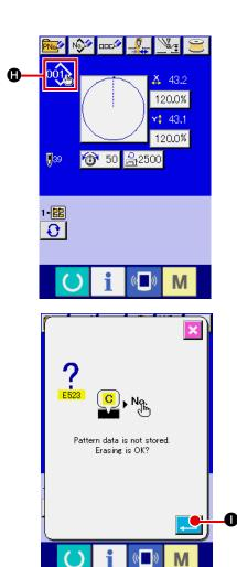
When X/Y enlargement/reduction ratio, thread tension, intermediate presser, adding/deleting of thread tension command, or adding/ deleting of increase/decrease value of intermediate presser of users' pattern or media pattern is performed, the pattern kind section becomes change display ().
