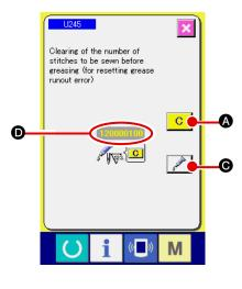
When the sewing machine has been used for a certain number of stitches, error "E220 Grease-up warning" is displayed. This display informs the operator of the time of replenishing the designated places with grease. Be sure to replenish the places with the grease below. Then call the memory switch U245, press CLEAR button
