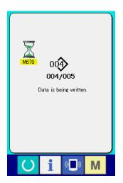
Data No. during communication, total number of writing data and number of data that have ended the data communication are displayed in the during communication screen.
