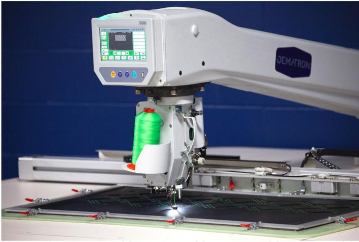
Large stroke needle rod mechanism and 22 mm needle height allow for different thickness of fabrics and versatility of sewing applications.
