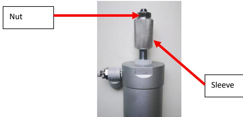
Loosen the fixing nut, rotate the limit sleeve, adjust the stroke of the cylinder, and change the indentation depth of the flower wheel.
