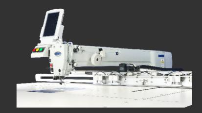
Sewing Speed 2,500 rpm Sewing Area 1000 mm. x 750 mm. Scavenging device Standard facility Thread Clamping device Variable tension of multi segments Cutting device Circular cutting knife Foot pressure Auxiliary presser foot + medium presser foot Press Foot height 20 mm. Hook Heavy material standard hook
