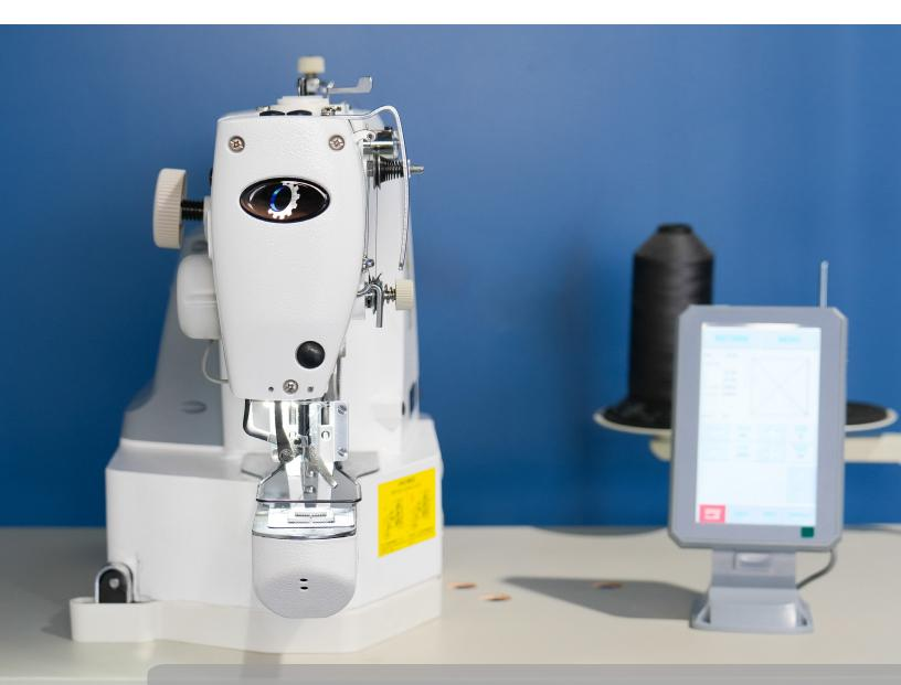
The Dematron DM-430S is upgraded with Direct-Drive Motor and 7" touchscreen to deliver added flexibility and versatility.
